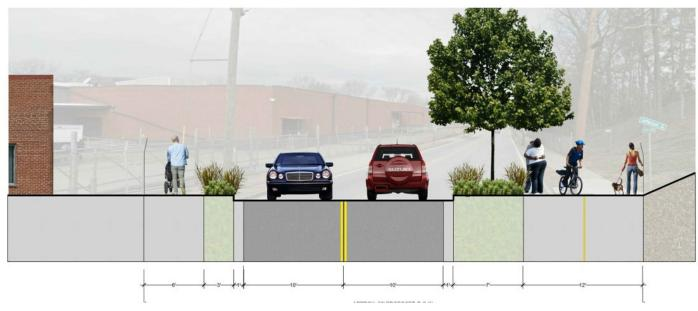
Cross-section: Section - Proposed Conditions on J.E. Lowery Boulevard (Option A) Source: the Collaborative, Inc.
