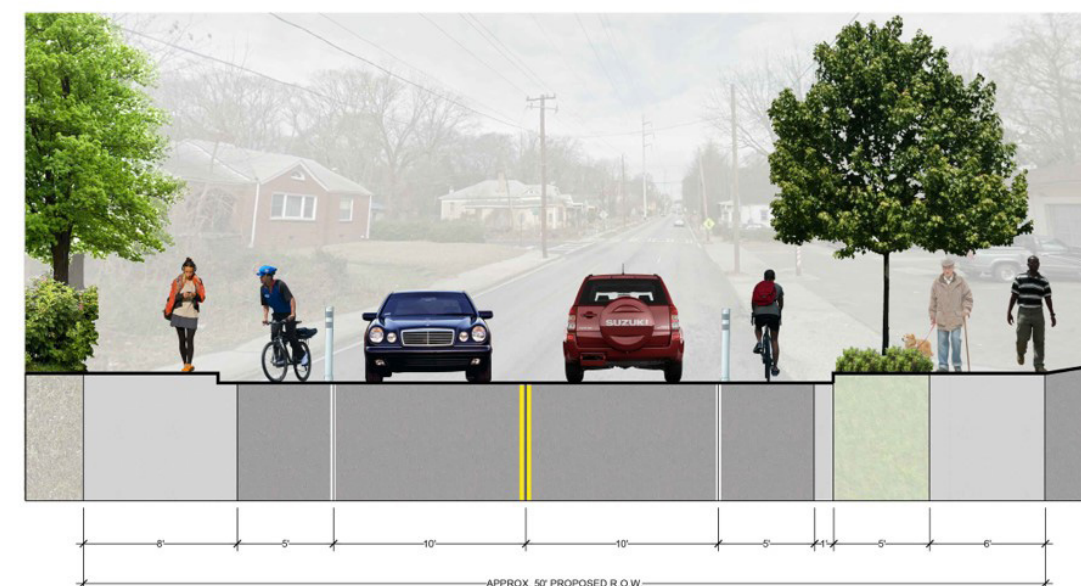
Cross-section: Proposed Conditions on J.E. Lowery Boulevard (Option A) Source: the Collaborative, Inc.
