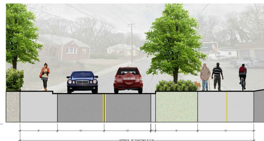
Cross-section: Proposed Conditions on J.E. Lowery Boulevard (Option B) Source: the Collaborative, Inc.
