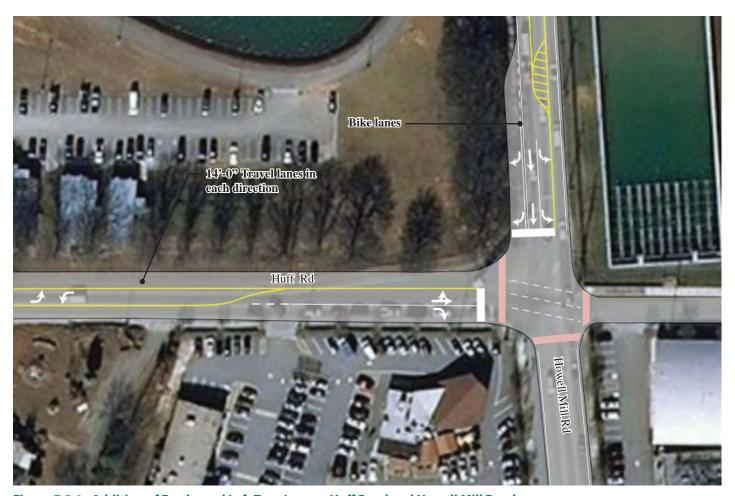
**Figure 7.2.1: Addition of Eastbound Left Turn Lane at Huff Road and Howell Mill Road** Source: AECOM
