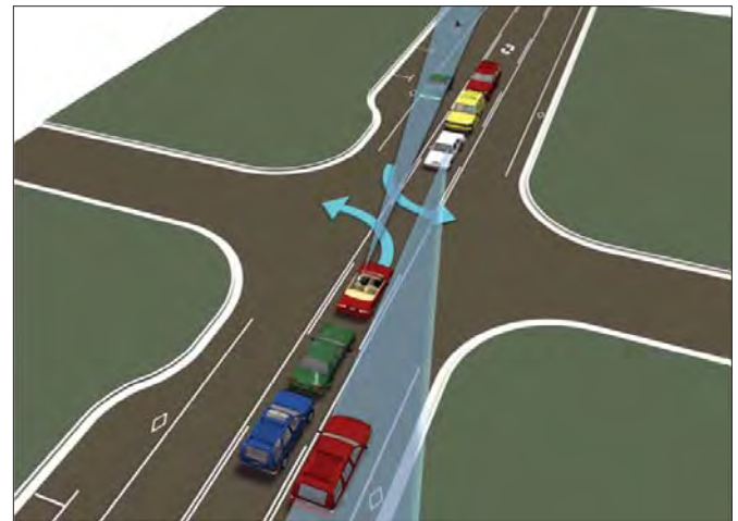
Figure 1.2.2 - Visibility associated with left hand turns on a 3-lane road.
