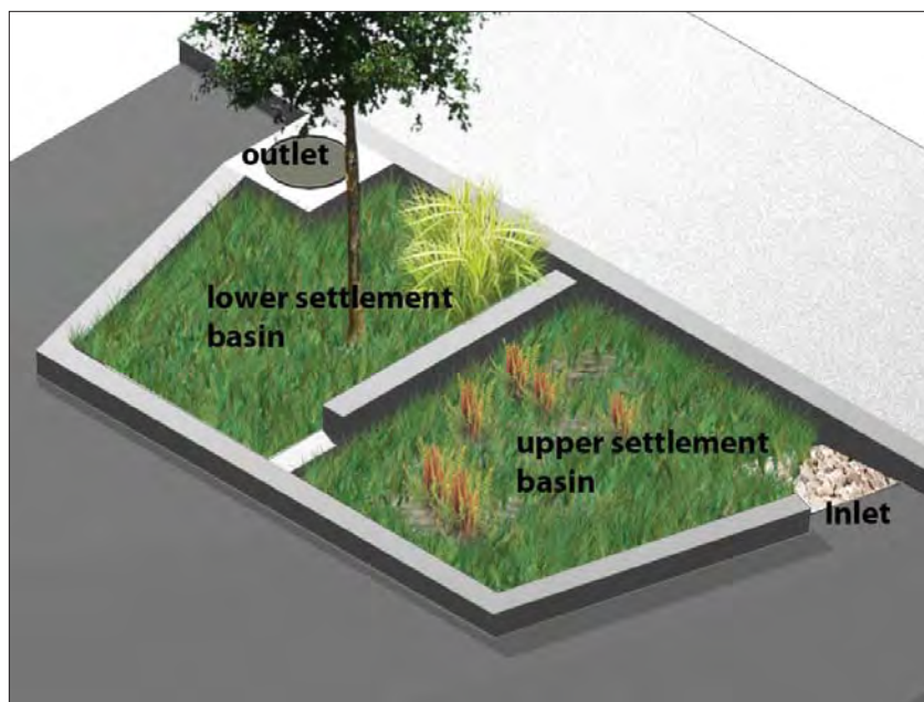
Figure 7.3.1 Bioretention Streetscape Enhancements
