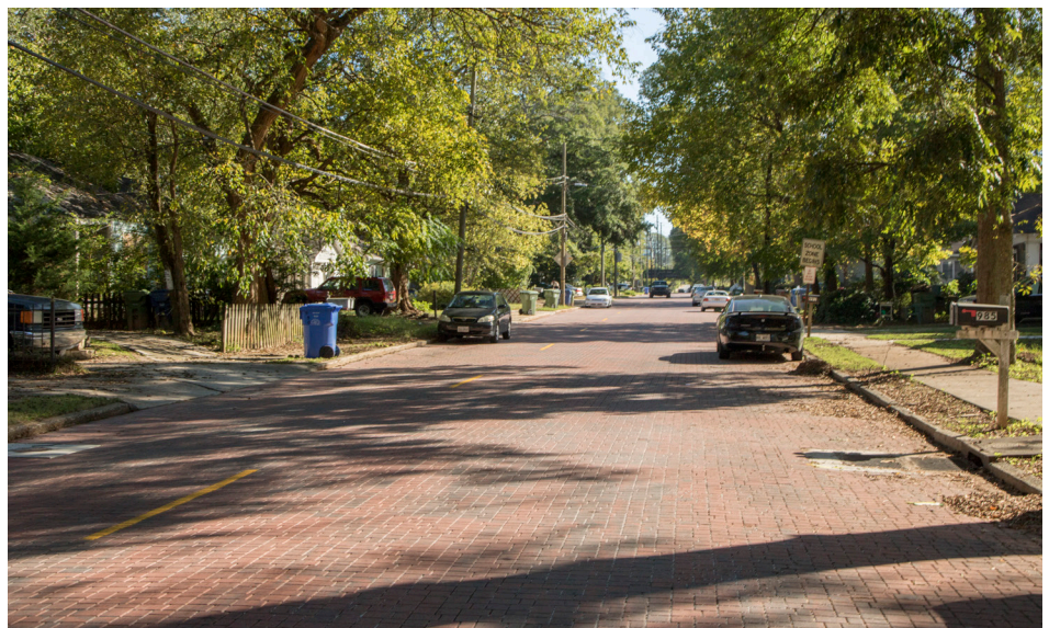
Improvements on major streets will provide safer access to the Atlanta BeltLine for pedestrians and bicyclists. Traffic calming measures, like permeable pavers on Hill Street shown above, can also contribute to stormwater management.
