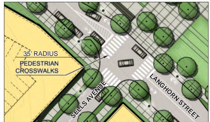
One possible reconfiguration could use a 35-foot curb radius for trucks turning from Langhorn Street onto Sells Avenue
