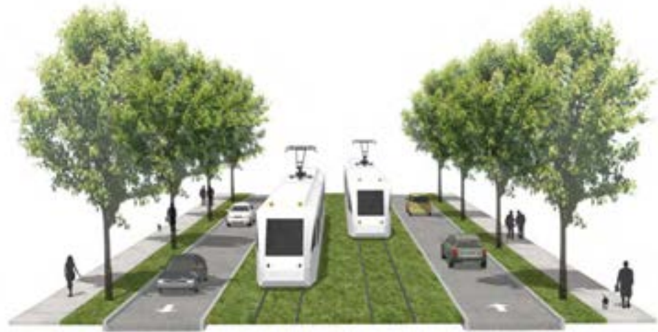
S2.5.2 CENTER: Transit in median; Trail in separate alignment
