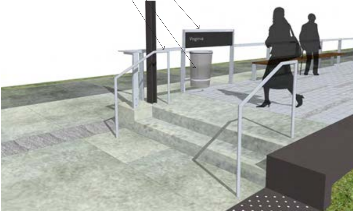
INTEGRATED STATION IDENTIFICATION SIGNAGE INTEGRATED RECEPTACLES FOR TRASH AND RECYCLING 36" STAINLESS STEEL HANDRAIL
