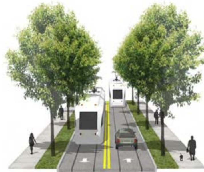
S2.5.3 SPLIT: Transit in mixed traffic; Trail in separate alignment
