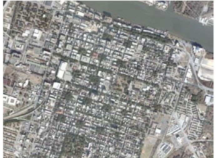
Many successful cities are based on flexible grid street systems that allow for change over time, such as Savannah
