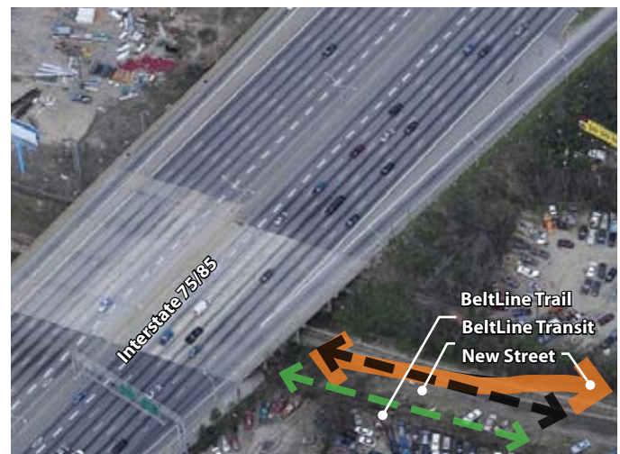
Underneath Interstate 75/85, there is room for a new street that would share space with BeltLine transit and trail
