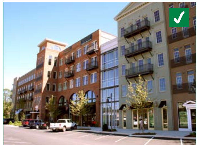
This single building in Woodstock, GA, creates interest with facades that truly resemble separate buildings, each with its own material, composition, and style
