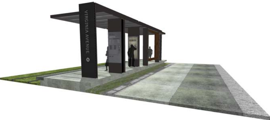
Transit Station Typology - The station canopy has thin-film photovoltaics for on site energy generation.
