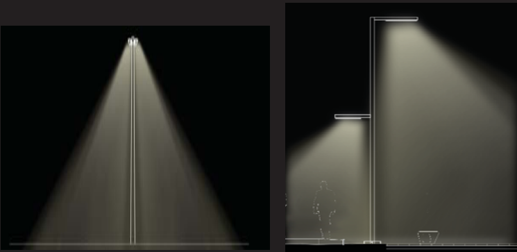
Alternative methods of guideway lighting: Flood pole (LT1.4) and Dual-level pole (LT1.2)
